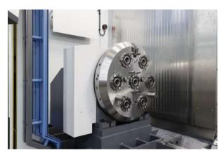
Rotary table RTA 5 as counterbearing with 7 zero point clamps in reinforced version
